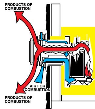
Empire's Direct-Vent wall furnaces are ideal where existing flues or chimneys cannot be used. Just one hole through an outside wall is all you need. If you must vent, you will receive maximum fuel economy from Direct-Vent heaters.
