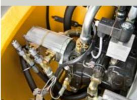
Separate working and steering hydraulic pumps.
