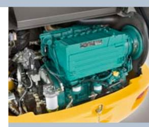
High-performance, 4-cylinder Volvo diesel engine.
